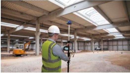
Racelogic is launching a brand-new indoor positioning system, called VIPS, which is an advanced system for measuring real-time 3D position to an accuracy of  $\pm 2\text{cm}$  in areas where GPS is not available, making it an ideal tool for construction applications both indoors and in urban areas. The system has been designed for any application that requires accurate measurement and recording of 3D positioning and enables GPS based technologies to operate in GPS denied environments.
