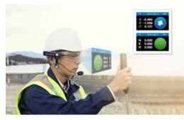
Topcon Positioning Group has introduced the LN-100 hands-free, voice-activated heads-up display (HUD) solution. This wearable assistant provides visual layout directions via HUD glasses that guide the operator using an <u>LN-100</u> to efficiently perform layout work at a construction site. The wearable assistant enables customers to use both hands to accurately mark layout points.
