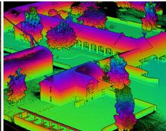
The pointclouds above were created by georeferencing the raw data from a LiDAR sensor with the inertial measurements from an OxTS INS. The bridge survey was conducted using a drone and the road and building survey data was collected on a mobile mapping vehicle (car).
